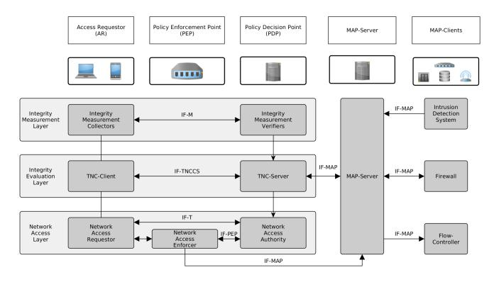
Figure 1. TNC architecture including IF-MAP, layers and 802.1x components based on [2, 13]
